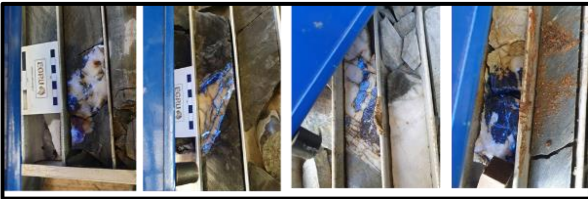
Figure 19: Core Showing Late Replacement of Wolframite by Fine Network Retrograde Scheelite
